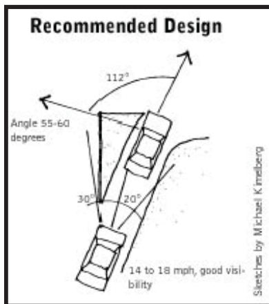
FIGURE 3.1.13 Modified Channelized Right Turn
